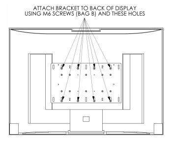
Figure 7. Display with 300mm x 200mm Hole Pattern
